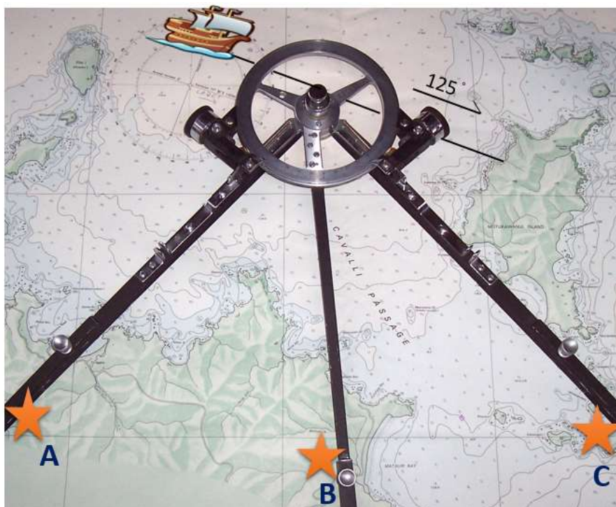
Figure 2.7. Fixing the ship using station pointer. Source: https://www.google.ro/search?q=station+pointer&source=lnms&tbn=isch&sa=X&ved=0ahUK Ewji8teLkMPUAhWkYpoKHfVUCkkQ_AUICigB&biw=853&bih=394&dpr=2.25#imgsrc=mgeL0p_482d8SM .
