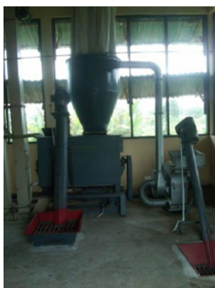
Figure 4: Mixer unit which is used in mixing feed ingredients homogeneously.
