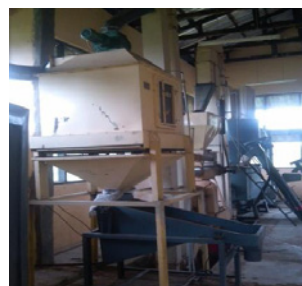
Figure 8: Cooler and feed collection unit where freshly pelleted feed is cooled and collected.
