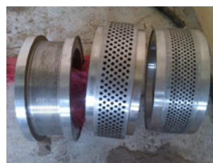
Figure 7: Di-rings used in the pelletizer for pelletizing feed to sizes ranging from 2 mm, 4 mm, 6 mm and 8 mm.
