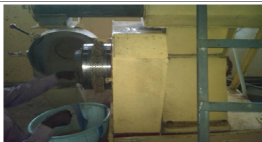
Figure 5: Pelletizer used in pelletizing feed to various sizes (2 mm, 4 mm, 6 mm and 8 mm).
