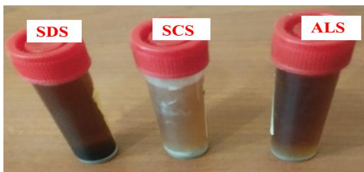
Fig 8. The stability results of nanofluids after 48 hrs for 0.5 wt% of G-FQDs with a ratio of 1:0.2
