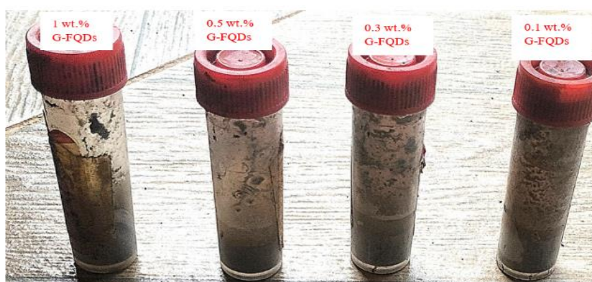
Fig 10. Stability results after 6 months of nanofluids at different G-FQDs concentrations with a ratio of 1:1.0 (C:S) using SDS surfactant
