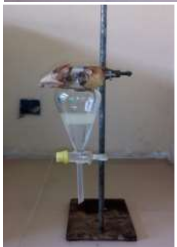
Figure 1: (a) Separated phased KSOME and glycerol. (b) Purified KSOME phased with water underneath.
