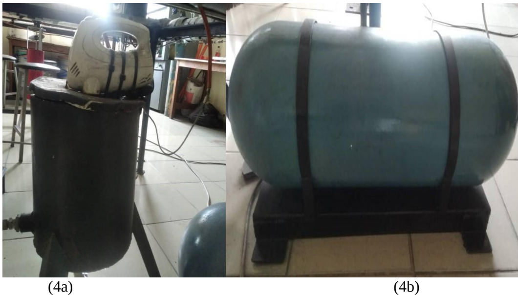
Figure 4. (a) Mixing chamber for water and percentage composition of hydrate inhibitor, (b) CNG cylinder composed of gas with weight 14g and specific gravity of 0.5
